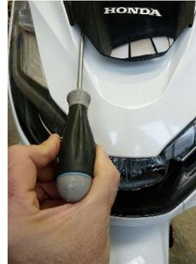
Remove the front molding by unscrew the two self-tapping screws located under the tip of the original windshield.
