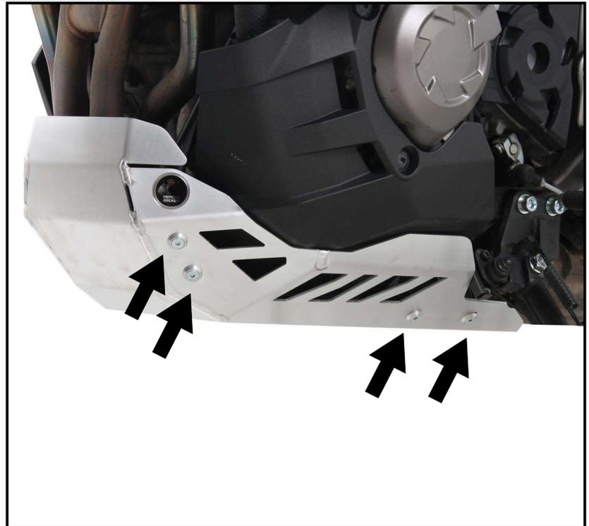
**Control all screw connections after the assembling for tightness!**
