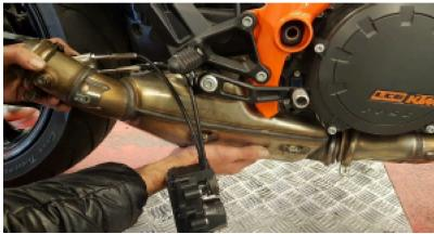
$\left( d\right)$  Remove trains and the plate of the actuator. To do so please secure disk
