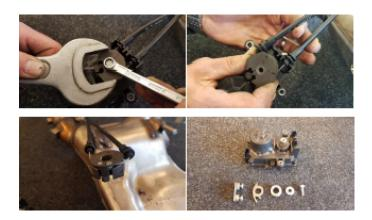
Install the BODIS stop in the subsequent order, and tighten.
