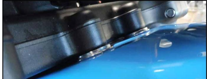
In combination with high fenders, insert the body washers Ø6.4xØ18 between the fender and frame. (see Fig. A)
